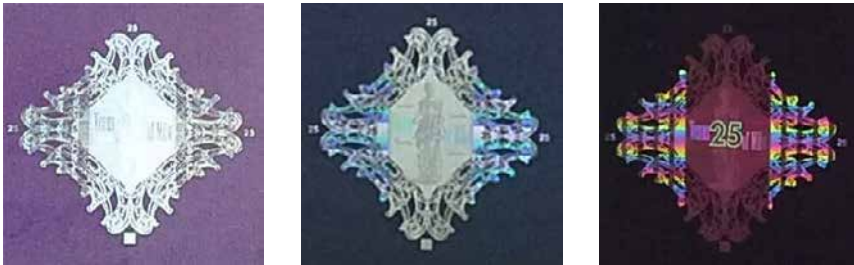
Figure A.12: Photograph of OVD13 under three different viewing angles. It is a Chromagram taken from [30] (Figure A.15.II). The paper is coated with Optically Variable Adhesive (OVA), which gives it a matte metallic appearance.
