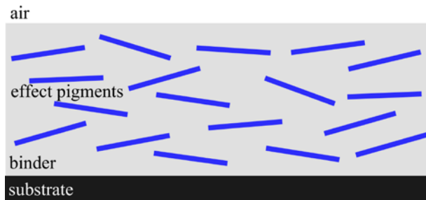
Figure 2.2: Schematic representation of a coating with special effect pigments. Some coatings can have an additional layer on top for increased protection from the environments.
