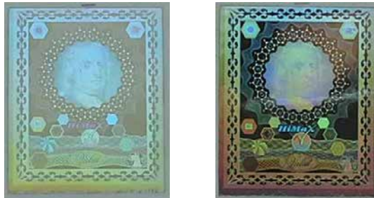
Figure A.9: Photograph of OVD10 under two different viewing angles. It is a HiMax OVD taken from [30] (Figure A.8) that consists of diffraction gratings with a width of 200 nm, "nanotext" and "nanologos".
