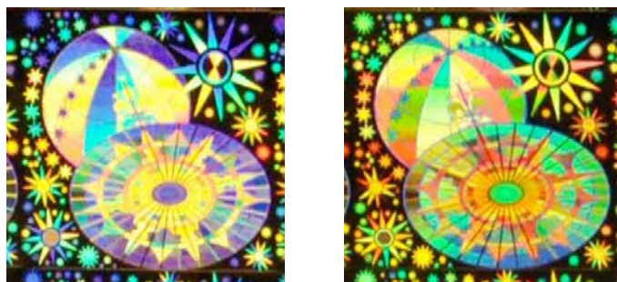
Figure A.14: Photograph of OVD16, an embossed reflective hologram foil, under two different viewing angles.
