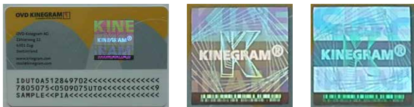
Figure A.7: Photograph of OVD8 under three different viewing angles. It is a Kinegram Secure Memory Card taken from [30] (Figure A.5). It allows straightforward first-line visual authentication.
