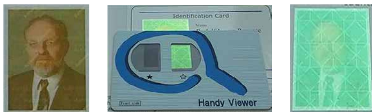
Figure A.3: Photograph of OVD4, taken from [30] (Figure A.14). It is a see-through diffractive interferential optically variable image structure, laminated over the portrait of an identification card. There is a color-shifting effect from transparent to green. The OVD4 was also photographed with the Handy Viewer that has left-handed and right-handed circular polarizers in the left and right openings, respectively. The sample is fully transparent through the left opening, while diffractive and interference effects are seen through the right opening.
