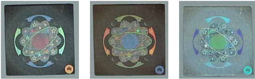
Figure A.5: Photograph of OVD6 under three different viewing angles. It is a Vectorgram taken from [30] (Figure A.3) made with electron beam lithography. It consists of an array of pixels in which each pixel contains two or more subpixels with different optical effects.
