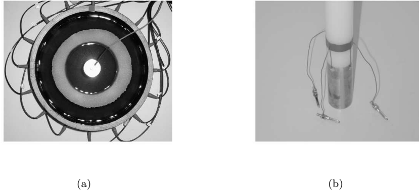
Figure 6.4: The experimental arrangement. (a) The two-dimensional tank with 16 boundary electrodes. In the center of the tank there is also a grounded stainless steel electrode. The foam plastic ring is also in the tank. (b) The central rod with four internal electrodes.
