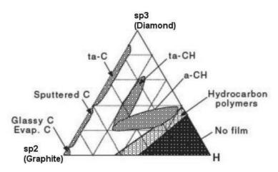
**Figure 4.2:** Phase diagram for various DLC films with respect to their sp<sup>3</sup> and sp<sup>2</sup> and hydrogen contents. (Modified from [134].)
