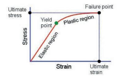
Figure 2.3: Fundamentals of bone's stress - strain curve under compressive loading.
