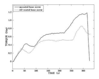
**Figure 7.1:** Insertion torque for two bone screws of diameter 2.7 mm, one with and one without coating. This test was applied to bovine femoral bone, which is significantly harder than human bone.
