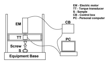
Figure 6.3: Schematic illustration of the developed test equipment for torque measurements.
