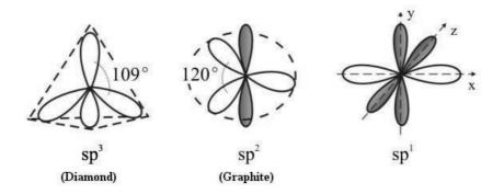
Figure 4.1: States of carbon bonding. (Modified from [134].)
