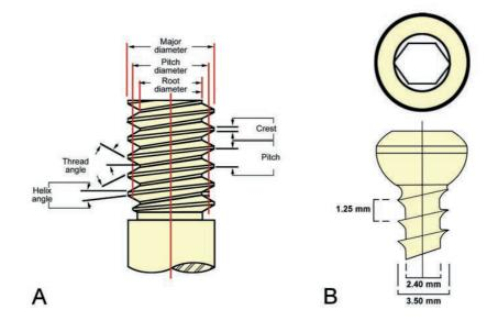
**Figure 3.1:** A) Screw anatomy with definitions. B) Dimensions of cortical bone screw used in the present study. (Modified from [53].)
