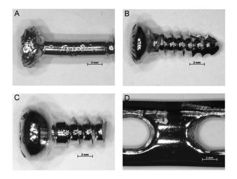
**Figure 3.4:** Stainless steel fracture fixation screws retrieved from patients indicating various defects on screws. A) Defects caused by removal tools. B) Tissue residue and deformation inducing different types of corrosion. C) Screw which was fractured during removal and D) Fixation plate showing *e.g.* marks of deformation.
