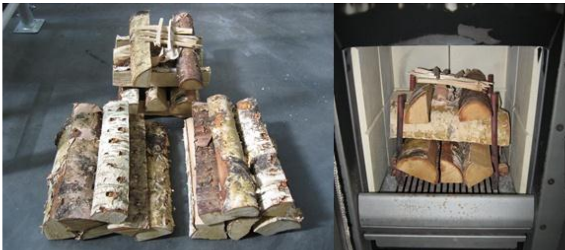
Figure 2. The wood fuel batches. On the right is the ignition batch placed into the furnace.
