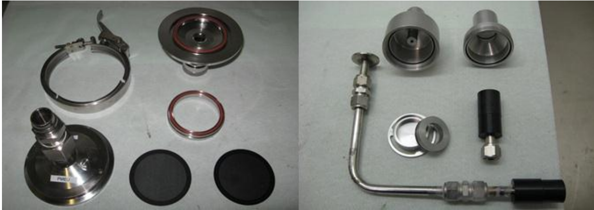
Figure 6. Filter holder and PM 2.5 separator used in the novel sampling method.
