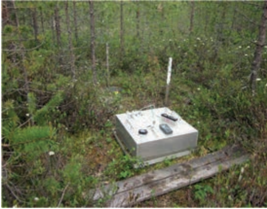
Figure 3. Static chamber measurement to analyze N 2 O flux.
