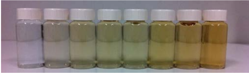
Figure 5. The lake and mire runoff water samples in 20 mL glass bottles, in the lake water mixing experiment (II). From left to right the bottles contain: milli-Q water, lake water sample (Kovero), mire and lake water mixture samples, mire runoff water NatB, ResB3 and ResB1 samples (respectively).
