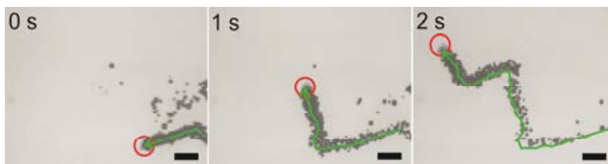
Figure 9. Time-lapse optical images of the autonomous propulsion of \text{MnO}_2 micromotors in 5% \text{H}_2\text{O}_2 and 0.1% SDS.
