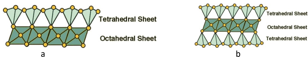
Figure 2. 1:1 (a) and 2:1 (b) clay structures 5
