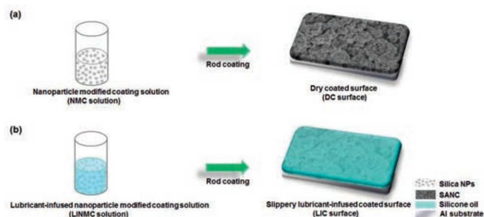
Figure 17. Processes for fabricating (a) dry-coated and (b) slippery lubricant-infused coated surfaces. The schemes are not drawn to scale.
