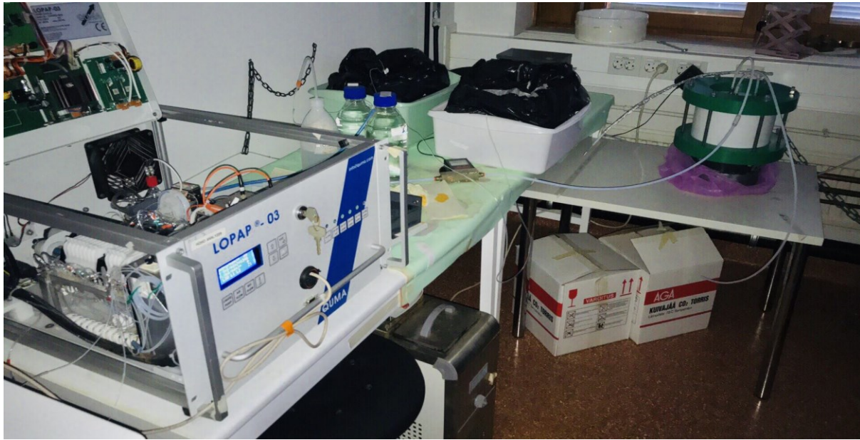
Figure 15: HONO measurement set up with the LOPAP device
