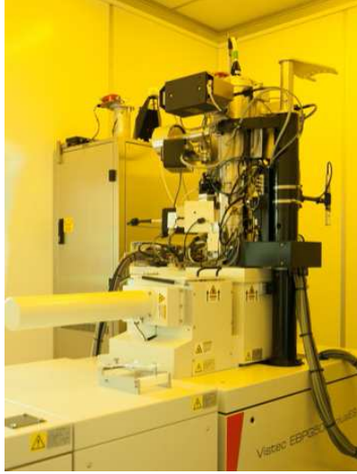
Figure 2.4: Image of a 100 keV beam energy EBL Vistec for lithography.
