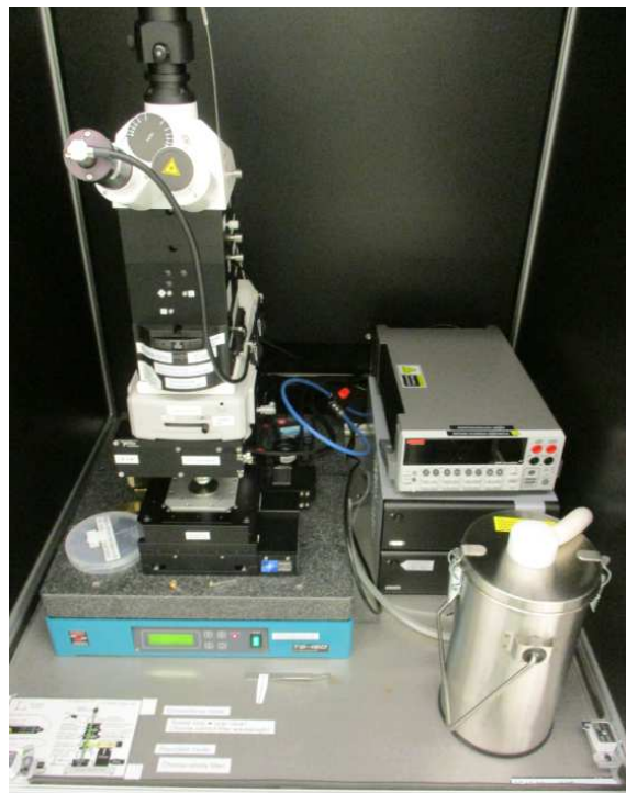
Figure 2.5: Image of a Linkam equipment THMS600 - heating and cooling stage.
