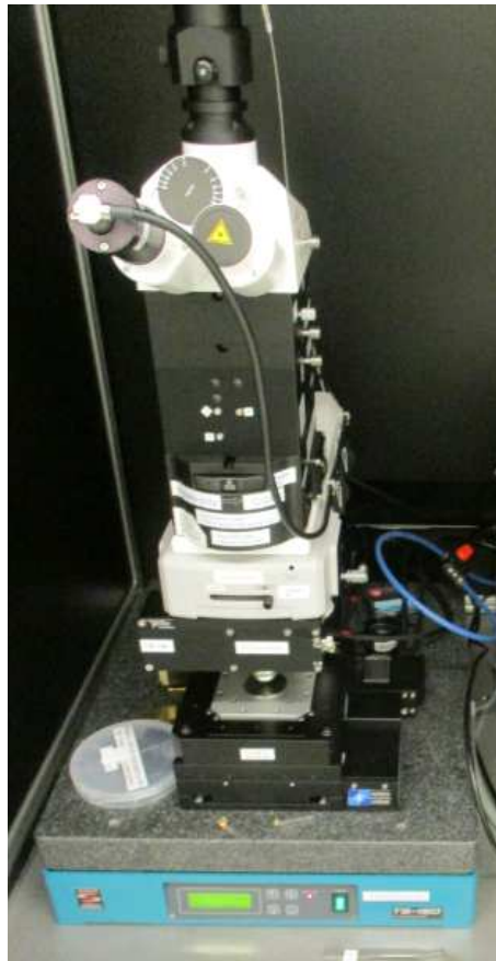
Figure 2.3: Image of a Micro-Raman used for Raman spectroscopy and optical characterization.
