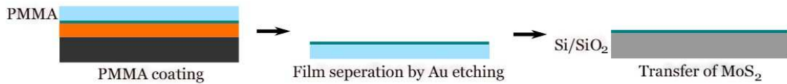
Figure 3.3: Transfer of two dimensional materials from M-Au sapphire substrate to the Si/SiO 2 substrate.
