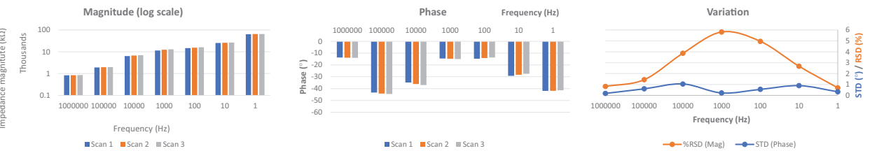
Figure 7. Impedance magnitude (left panel) and phase (middle panel) values at seven discrete frequencies (1 Hz to 1 MHz) in repeated BIS measurements (three scans) for cucumber sample. Inter-scan variation graphs (right panel) show relative standard deviation (RSD, %) of impedance magnitude and standard deviation (STD, °) of phase data. Data obtained with the 3D printed probe (upper part of figure) are shown in comparison to the concentric ring probe data (lower part of figure).
