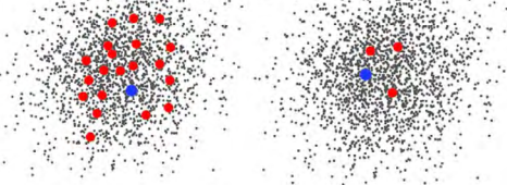
Fig. 5. Distribution of slope points (gray) and local peaks (red) inside an example cluster. One of the local peaks (blue) is the resulting cluster centroid (global peak). The case of k=30 (left) and k=70 (right) are shown. When the number of neighbors k in the kNN graph is increased, the number of local peaks decrease. (For interpretation of the references to colour in this figure legend, the reader is referred to the web version of this article.)
