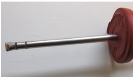
Picture C. Rubber disk set to first sampling depth.
