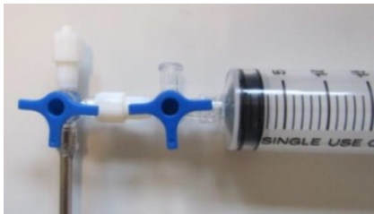
Picture B. Syringe connected to the gas probe.
