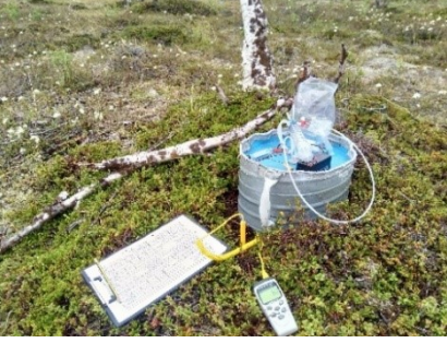
Photo 2. Chamber measurement set-up with field template and thermometer with soil probe.
