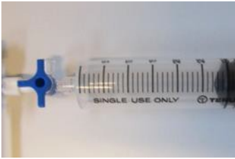
Picture A. Syringe with 30 mL of ambient air & closed 3-way valve.
