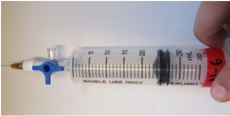
Picture M. Valve open, needle flushed with ~5 ml of sample.
