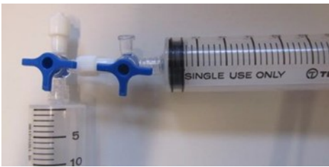
Picture J. An empty syringe connected to the syringe with the soil water sample.
