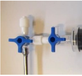
Picture G. Discarding the 1-2 ml of water before taking the soil water sample.
