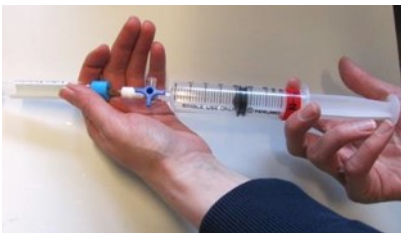
Picture N. Needle connected to vial, inserting 25 ml of sample gas to the exetainer.
