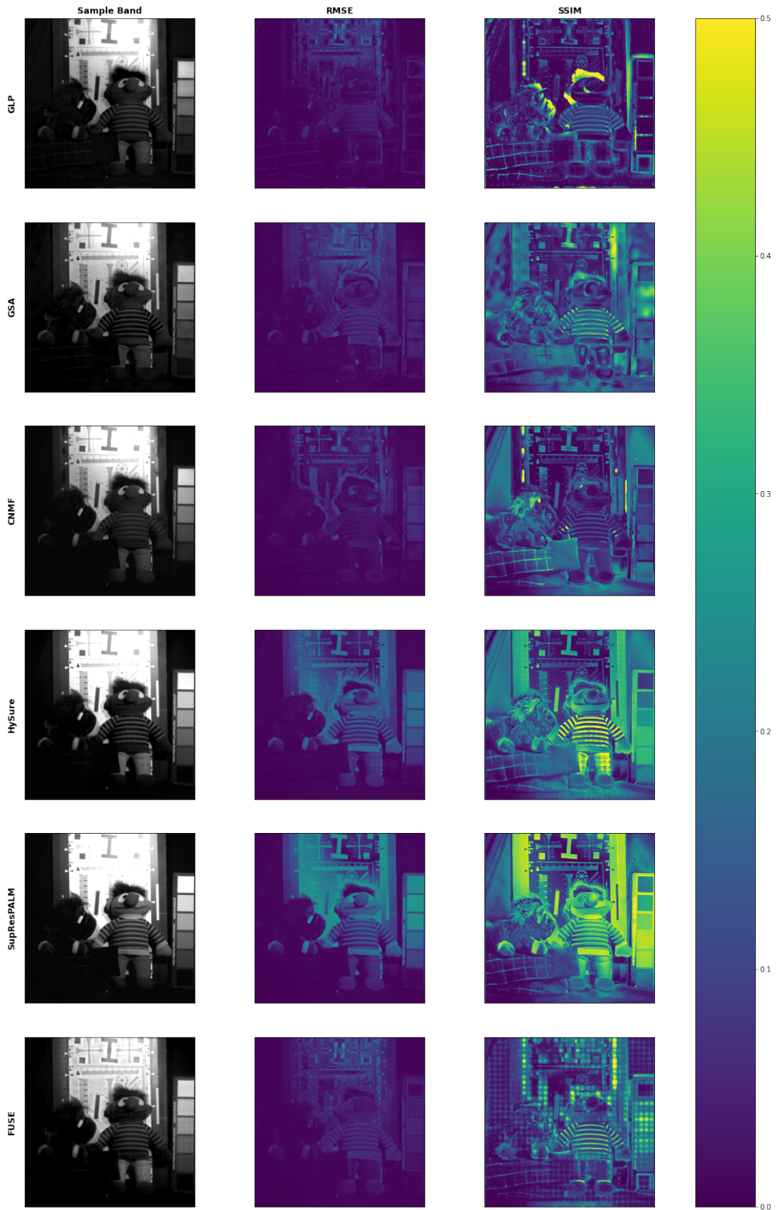
Figure 4.4: Visual analysis of RMSE and SSIM maps of the image "chart_and_stuffed_toy" from the CAVE dataset across different HIF methods with a scaling factor of 16x.
