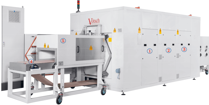
Figure 1.1: External view of the HEPHAISTOS microwave oven system. Main modules of the oven that contains high power microwave waveguide antenna are represented by numbers tags 1, 2, and 3. Tag 4 is the conveyor belt used for continuous processing of material. Tag 5 represents the microwave filter which is used for blocking leakage power. Picture courtesy of Weiss Technik GmbH, Germany.
