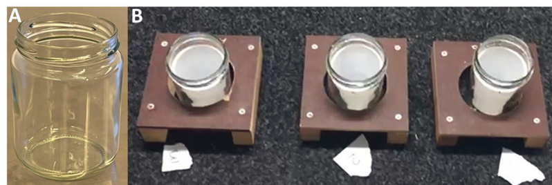
Figure 2. Individual plywood stands were used in Study 3 as a three-alternative forced-choice device (A); glass jar (B); glass jars containing the plastic cup with target or non-target sample.
