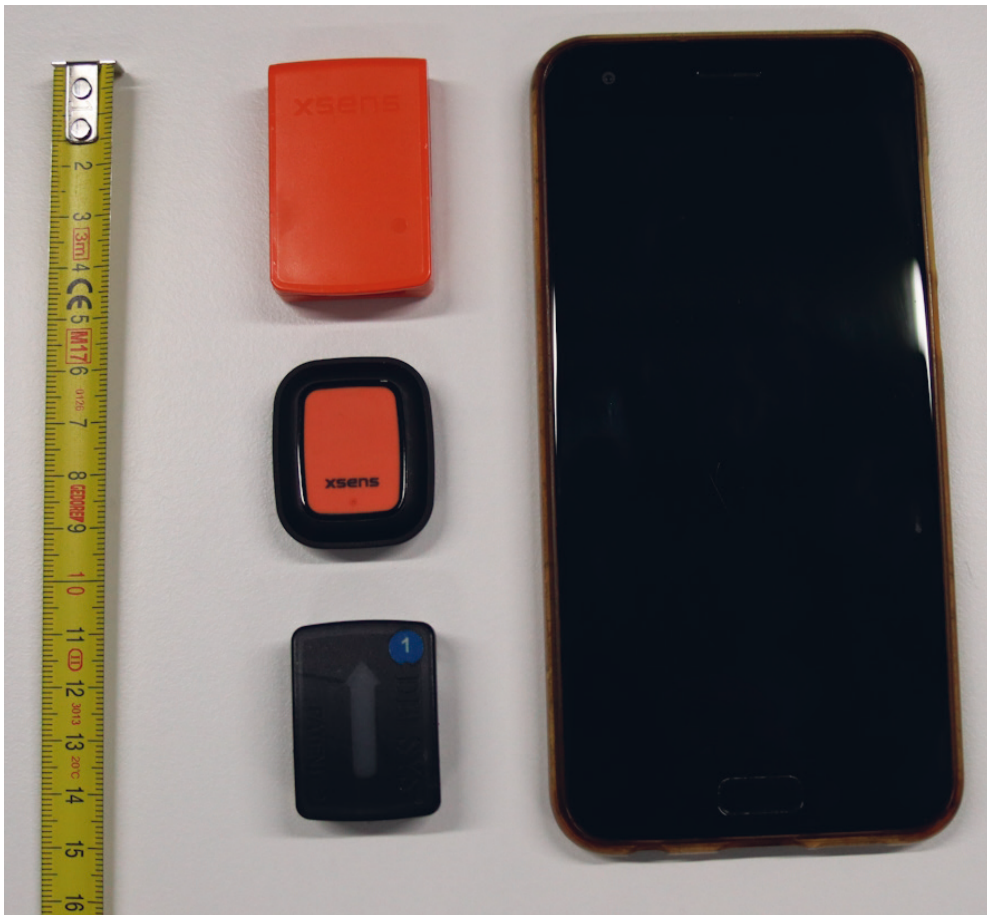
Figure 3.4: Wearable devices that can be used in motion capture include inertial measurement units and even smartphones. Inertial measurement units are particularly useful as portable modalities to measure motion due to their small size. The three devices on the left of the smartphone are inertial measurement units, with the bottom-most also including electromyographic sensors.
