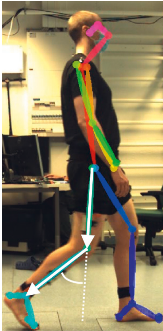
Figure 6.14: Knee flexion angle at each frame can be estimated by calculating the angle between the vector from the hip keypoint to the knee keypoint and the knee keypoint to the ankle keypoint. The vectors are drawn in white.
