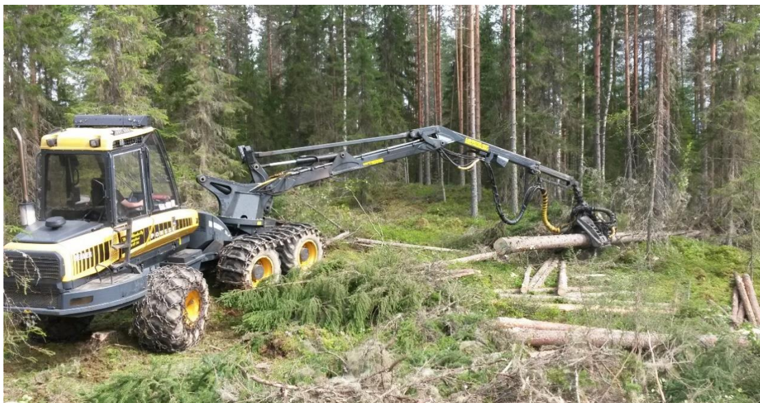
Fig. 2. Log bucking in the study with the Ponsse Beaver harvester in a spruce-pine-mixed stand. Photo: Jyri Änäckälä..
