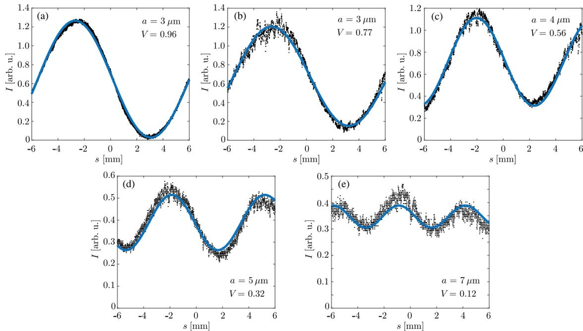
**Fig. 2.** Illustration of the far-field intensity patterns averaged over several measurements (black dots) and fitted curves (blue solid lines) as a function of the detector position  $s$ . (a) Scaled-down (focused) single-mode laser beam when the particles are  $3 \mu\text{m}$  apart. (b)–(e) Scaled multimode laser beam when the particles are separated by a distance of  $a = 3, 4, 5,$  and  $7 \mu\text{m}$ , respectively.
