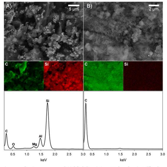
$\label{eq:Figure 4. Energy dispersive x-ray spectroscopy analysis including backscattering images (top), elemental mappings (middle) and elemental spectrums (bottom) of the (A) nSiC/C composite and (B) graphene-like carbon.$
