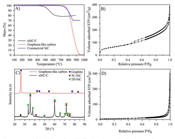
**Figure 2.** (A) TGA curve of nSiC/C before annealing, graphene-like carbon and commercial SiC after induction annealing, (B) Nitrogen adsorption-desorption isotherm of nSiC/C and, (C) XRD diffractograms of nSiC/C composite and graphene-like carbon and (D) Nitrogen adsorption-desorption isotherm of graphene-like carbon produced by induction annealing of nSiC/C.
