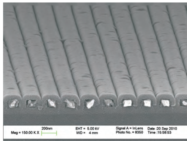
Fig. 2. Cross section of the absorbing polarization filter corresponding to the design A. The sample was fabricated with electron beam lithography. The metal wires are aluminum and the surrounding material is atomic layer deposited titanium dioxide. The image is taken with scanning electron microscope.
