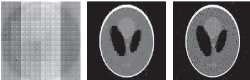
Figure 5.17: . L-curve method, S-curve method and Morozov discrepancy principle applied to data set with 37 projections. Reconstructions with selected alphas from left to right are: the MAP estimate with \alpha selected using the L-curve method \alpha_L = 33022 , the MAP estimate with \alpha selected using the S-curve method \alpha = 15.24 and the Tikhonov reconstruction with the \alpha selected using the Morozov discrepancy principle \alpha_M = 6.68 , respectively. The reconstruction resolution is 128 \times 128 .
