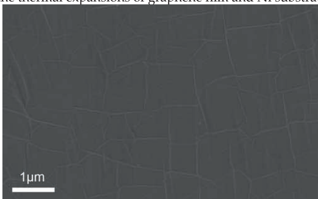
Fig. 11. SEM image showing wrinkled topology of few-layered graphene on a polycrystalline Ni substrate
