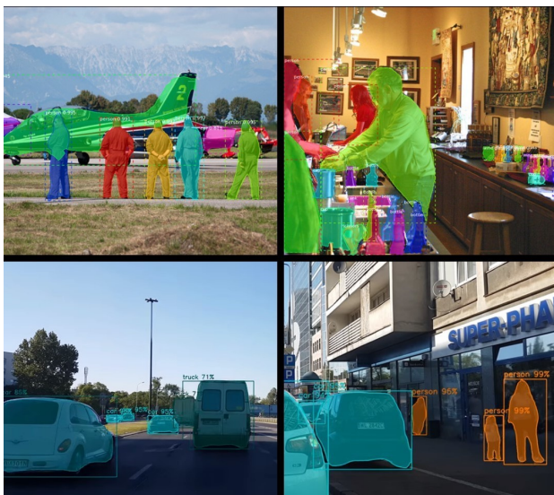
Figure 2. Mask R-CNN results on the COCO test set [24]. The results are based on backbone ResNet-101. The bounding box, category prediction, and class score are presented.
